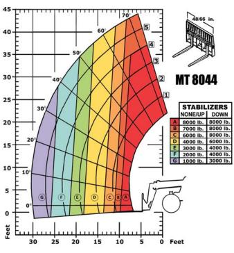
Capacities shown in pounds/feet are the maximum recommended load limits at the indicated extensions of the boom. Capacity ratings are based on a 48" homogeneous cube and are in accordance with ANSI/ASME B56.6 stability standards. Capacity reductions must be made for extended load centers and when used with various other attachments, contact MANITOU NORTH AMERICA, INC.
